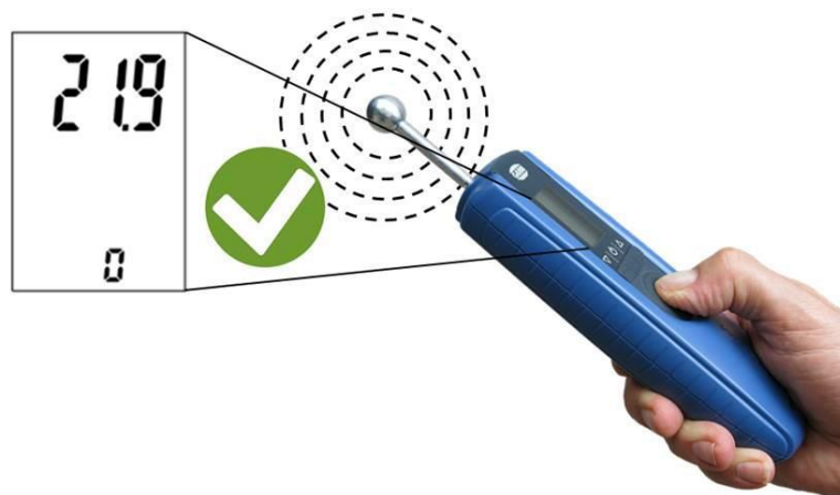
Figure 9-1: Correct device position
