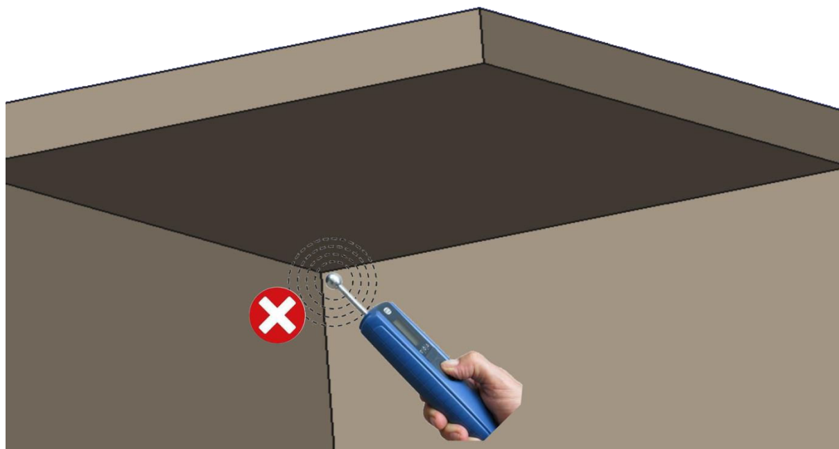
Figure 9-6: Incorrect use in corner/angle area
