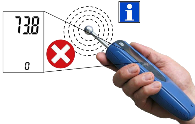
Figure 9-2: Improper device position
